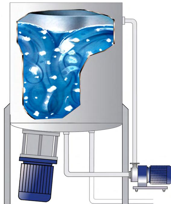
The solids are rapidly reduced to smaller pieces which are drawn into the interior of the workhead and subjected to intense shear before being forced out through the stator and back into the surrounding liquid.
