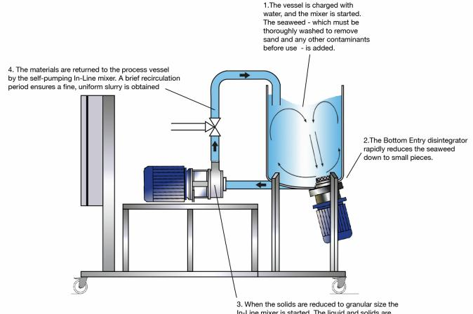
In-Line mixer is started. The liquid and solids are drawn into the workhead and subjected to intense high shear, which further reduces particle size
